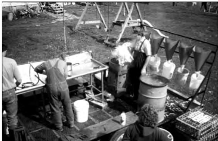
The Central NY Pasture Poultry Association’s mobile processing unit in operation. The man at right is standing between the scalding tank and plucker, with kill cones behind him.
